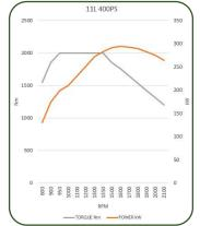
GH11TD460PS 338KW(460PS) @ 1,700rpm 2,250Nm (1659 lb-ft) @ 1,000 - 1,200rpm
